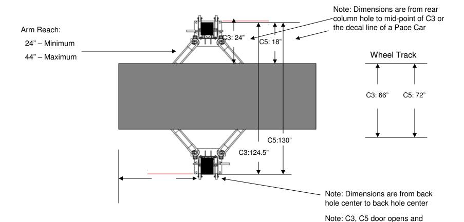
Note: C5 column location use 124.5" rearward anchors from C3 location. C5 lift location uses GM designated lift pads (see Page 2)
