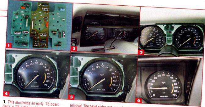
Inis illustrates an early '75 board (left), a '75-'76 board (center) and a 1977 board (right). Note the component counts (Boards courtesy of John Gardner).
