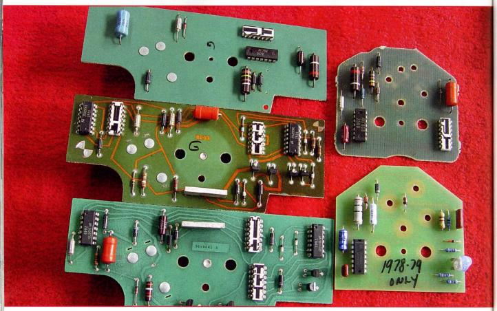
**ABOVE:** Four boards in this photo are original tach circuit boards installed in 1975-82 Corvettes, but only one is a restoration board. Which is a reproduction?
