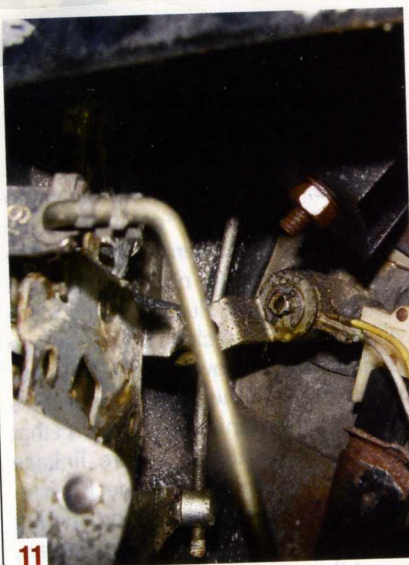
11 Removal of plastic guard reveals anti-theft lock cylinder & lock mechanism. Note the yellow and light-blue wire from the lock. Also note the film residue (yellowish) after cleaning.
