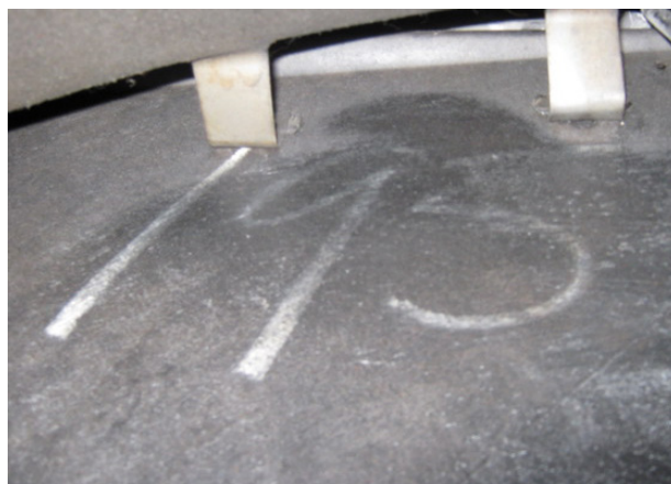
Figure 4a: Job Number 195 on a 1973 underbody panel
