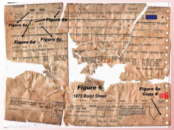
sheets were printed with the RPO data and destination data. The use of printed broadcast codes saw limited application. It is only speculation, but 1973 was a year of transition from Chevrolet Car Division management to the GMAD assembly plant management. The build sheet was introduced, but in all likelihood, the factory continued to use the methods that had been used during early C3 production, such as the chassis broadcast copy.
