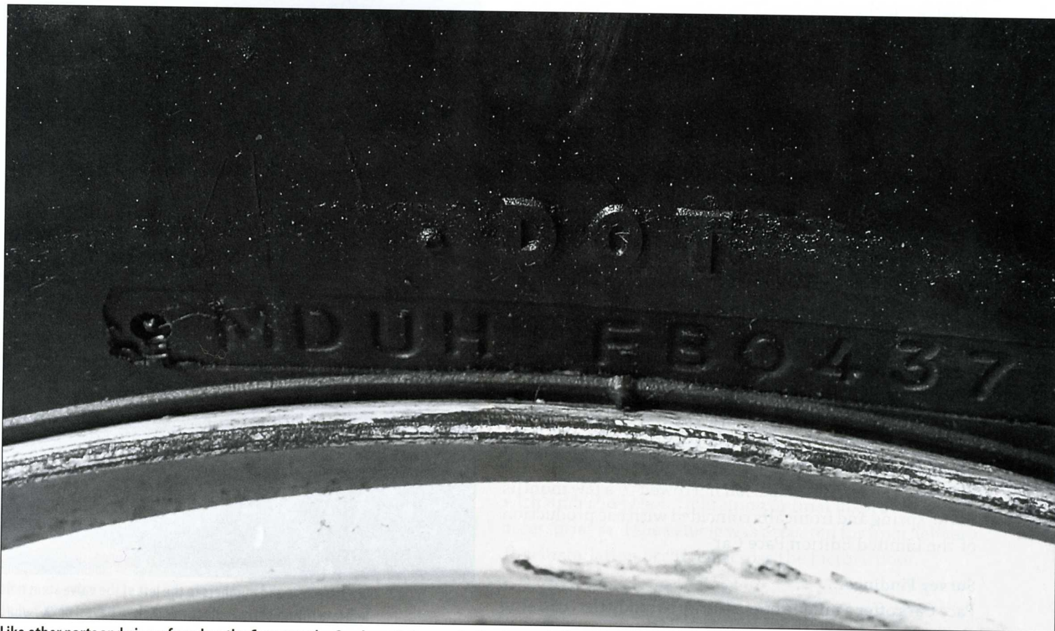
Like other parts and pieces found on the Corvette, the Goodyear Polyspare is also date coded. Here, VIN 9041 with a build date of November 10, 1977 reveals a Polyspare tire with date code of the 43 rd week or the week of October 24 th .
