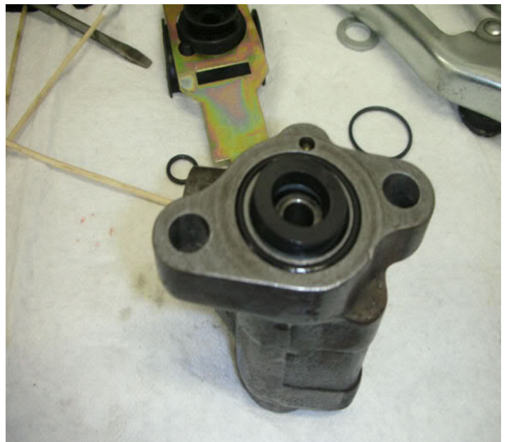
Figure 12: Valve housing with seal and o-ring
