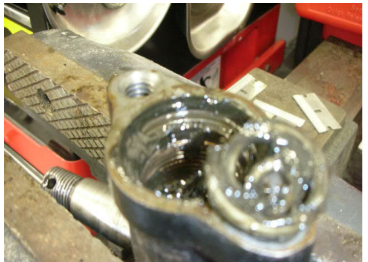
Figure 6: Housing, o-ring groove & ball seat spring
