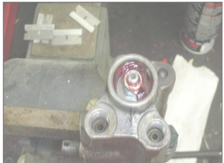
Figure 3: PSCV adjusting nut (dust cap removed)
