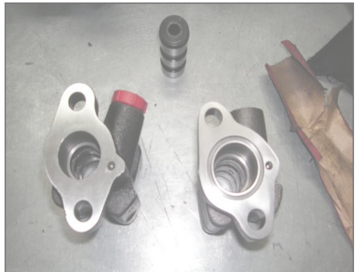
Figure 1: Valve housing smooth vs. o-ring groove
