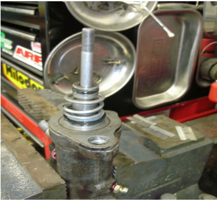
Figure 9: Valve reaction spool (piston) slides over valve shaft and inside the valve spring
