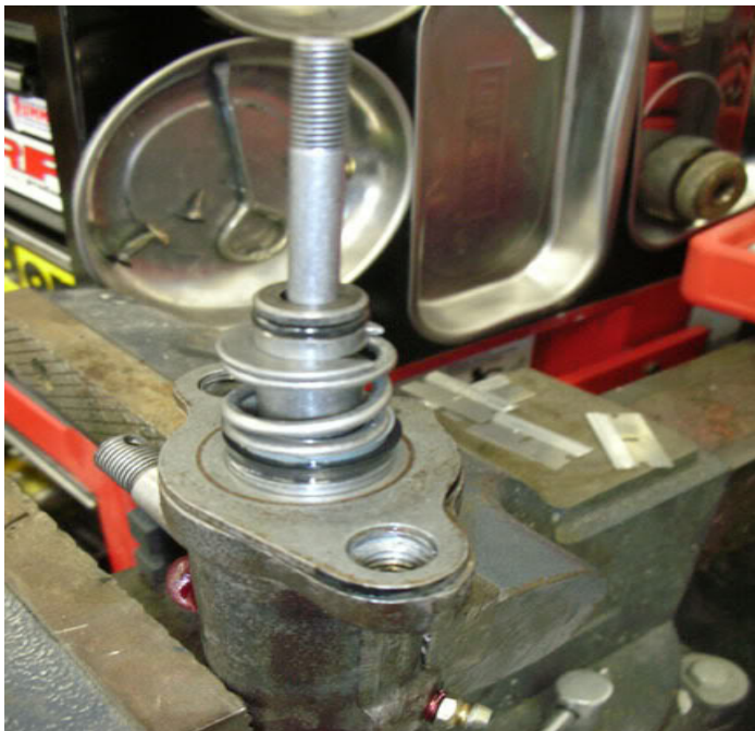
Figure 6: Ball stud side up with part stack assembly
