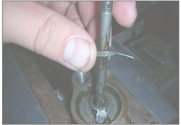
Figure 4: Valve shaft (rod), shaft washer & sleeve key
