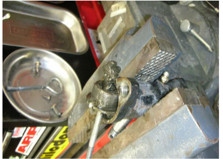
Figure 5: Rod removed with ball and adjustment nut
