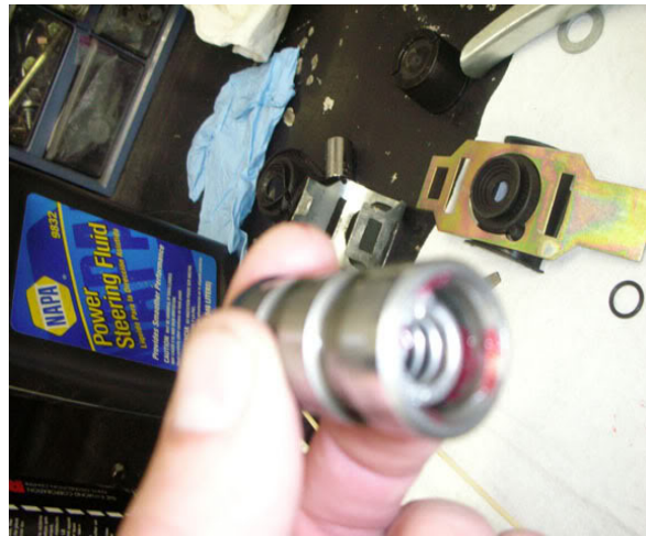
Figure 11: Valve spool & valve adjustment spring
