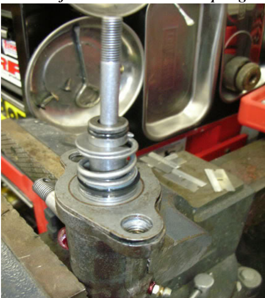
Figure 10: Spring thrust washer (keeper) inserts into valve spool and secures valve spring assembly
