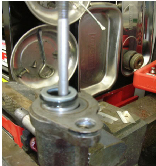
Figure 7: Spring retainer (top) and annulus seal
